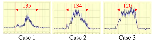
(b) Image processing examples of spray width measurement at 100 mm downstream from the nozzle exit with inlet air velocity, u_{in} = 5.4 \text{ m/s}
