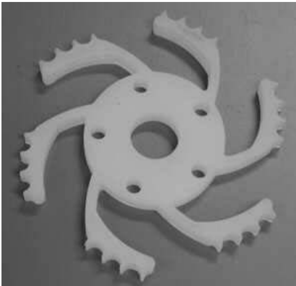
Figure 9: Independent arm CVT design
