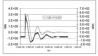
Fig. 3: Current and voltage waveforms used in the explosion test, leading to a peak power of about 110 MW.
