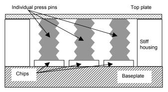
Fig 1: Schematic view of the pressure scheme used to decouple the external clamping force from the direct pressure on the chip. The contact partners on the chips (individual press pins) are flexible and upon clamping, they are compressed until the top plate and the base-plate touch the stiff housing material. When the external force is further increased, the pressure on the chips will remain stable whereas the housing will take the additional force.
