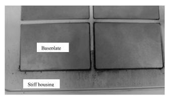
Fig. 4: Bottom side of the module, showing the base-plates as well as the stiff housing. Despite the peak power of 110 MW in the explosion test, the module housing is still intact.
