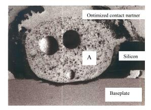
Fig. 2: The low melting compound (A), formed between the silicon and its partners, ensures a highly conductive and long term stable path through the chip.
