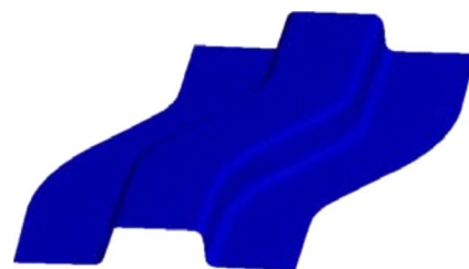
Fig. 14 Initial solution of intermediate configuration with 20 mm drawing depth
