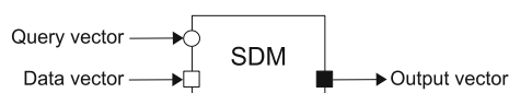
Fig. 2 Schematic illustration of a sparse distributed memory (SDM), which is an associative memory for random high-dimensional binary vectors [9]
