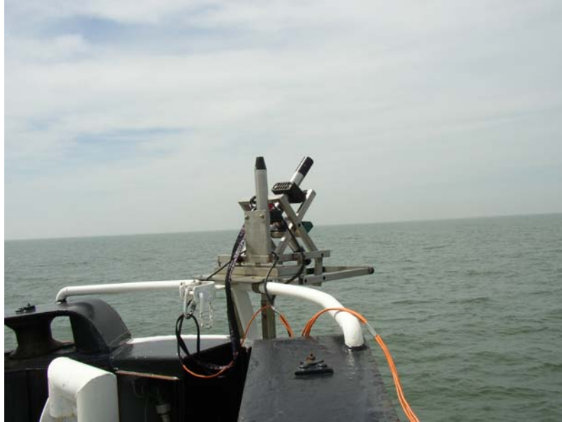
Figure 1 System of three spectroradiometers installed on a steel frame at the prow of the Research Vessel Zeeleeuw.
