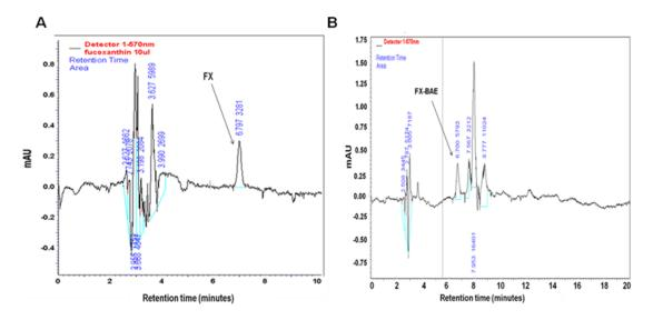
Figure 2. Chromatograms analysis of fucoxanthin-rich brown algae extract using HPLC. FX-BAE was obtained and compared with fucoxanthin standard by using HPLC. The condition of operation included: Colum RP-18, mobile phase (acetontrile : methanol : water; 67.5: 13.5 :19) containing 0.1% (w/v) ammonium acetate and flow rate of 1 mL/1 min. Chromatograms of fucoxanthin standard (Figure 2A) and X-BAE (Figure 2B) were indicated by the black arrow
