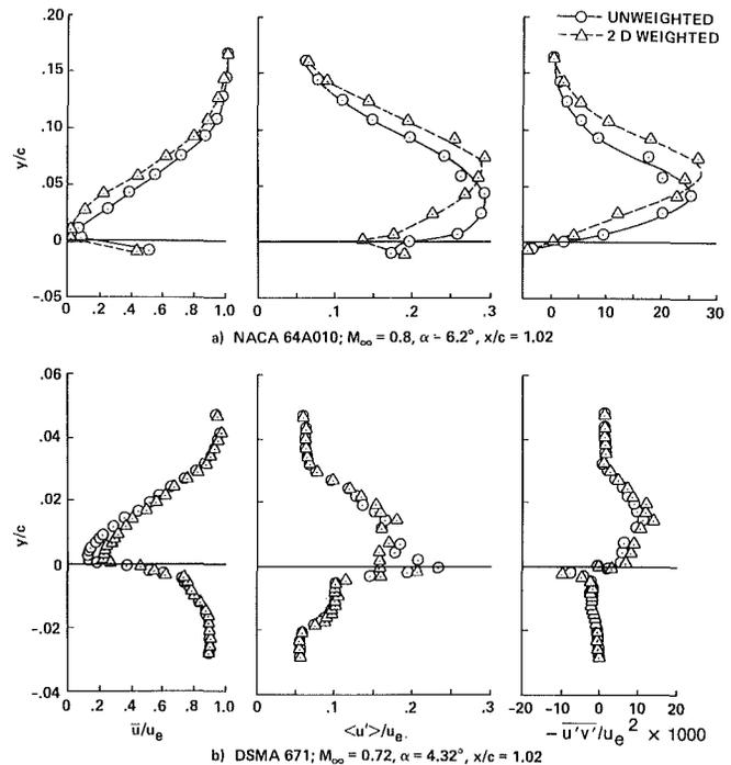
Fig. 11 Uncorrected and bias-corrected results; airfoil models
