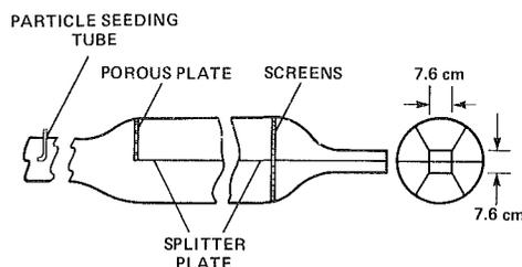
Fig. 1 Schematic of two-stream mixing flow model
