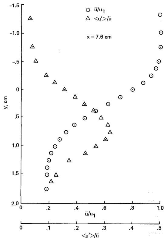
Fig. 2 Shear-layer mean velocity and turbulence intensity distributions
