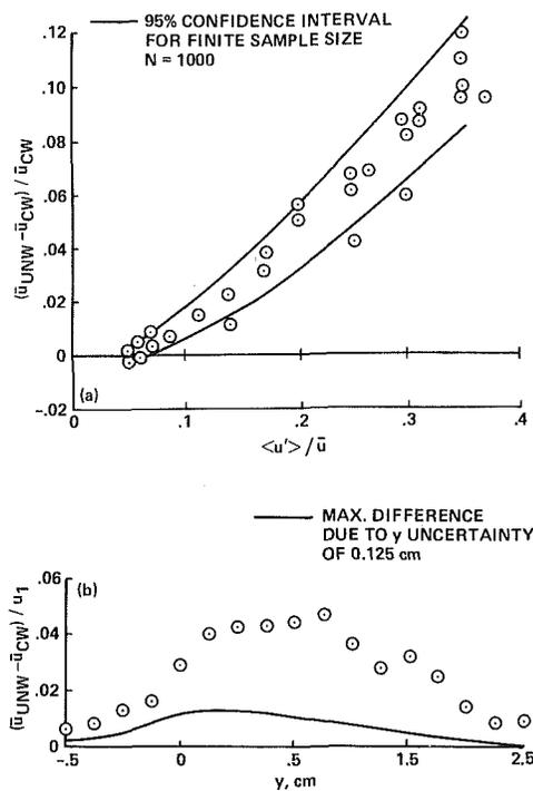
Fig. 4 Differences in continuous-wave and individual-realization (unweighted) mean-velocity measurements:
