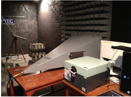
FIGURE 7: Under EMC test (IEC 60118-13).
