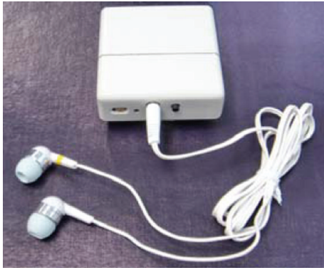
FIGURE 1: PDN-01B digital hearing aid developed.
