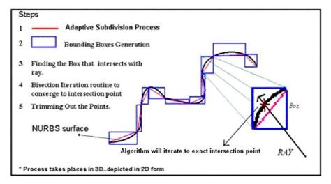
Fig. 5. Step by step procedure on calculation of NURBS intersection points.
