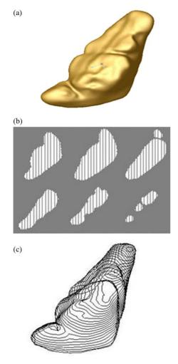
Fig. 9. (a) Case study example model 2—sinus graft 1 with 102 NURBS surfaces. (b) Slice raster lines at different slice layers. (c) Entry and exit points displayed.
