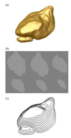
Fig. 10. (a) Model 3 sinus graft 2 layout—135 NURBS surfaces. (b) Slice raster lines at different slice layers. (c) Sliced entry and exit points displayed.
