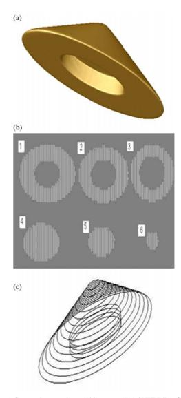
Fig. 8. (a) Case study example model 1—cone with 44 NURBS surfaces. (b) Slice raster lines at different slice layers. (c) Entry and exit points displayed.
