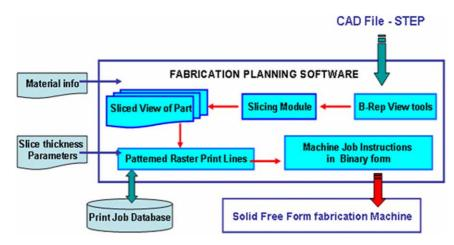
Fig. 3. Process flow during fabrication.
