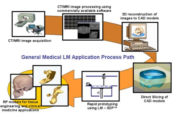
Fig. 2. General biomodeling and medical rapid prototyping process path.
