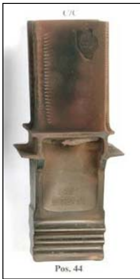
Figure 6: Typical TBC Coated 1 st Stage Blade After 7,192 Hours
