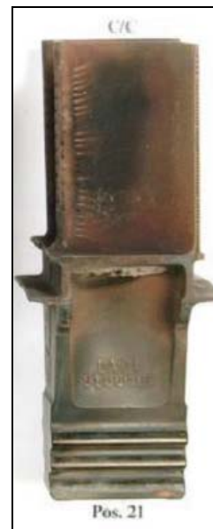
Figure 7: Typical SermaLoy J Coated 1 st Stage Blade After 7,192 Hours
