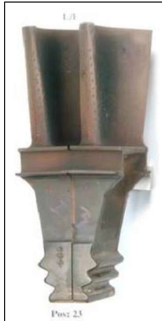
Figure 1: Typical PBC-22 Coated 1 st Stage HPT Blade After 7,192 Hours
