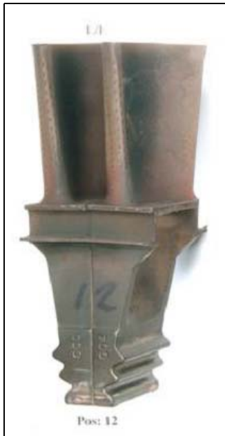
Figure 2: Typical BAJ BC-22 Coated 1 st Stage Blade After 7,192 Hours
