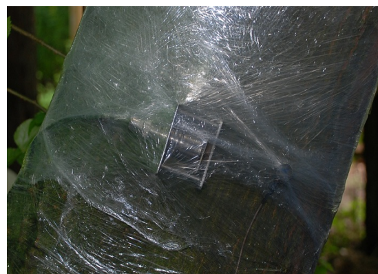
2: Placement of AE sensors on the tree on steel blade (a) and on waveguide (b) – left, final arrangement of test – right
