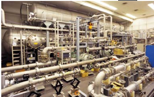
FIGURES 8. THE AIR FLOW FACILITY AT AIST EMPLOYED TO CALIBRATE THE ORIFICE FLOWMETER; THE LOWER TANK ON THE FAR SIDE IS THE CONSTANT VOLUME TANK AS THE NATIONAL STANDARD IN JAPAN
