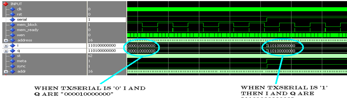
Fig. 18 Simulation Results of INPUT module (4-QAM modulator)
