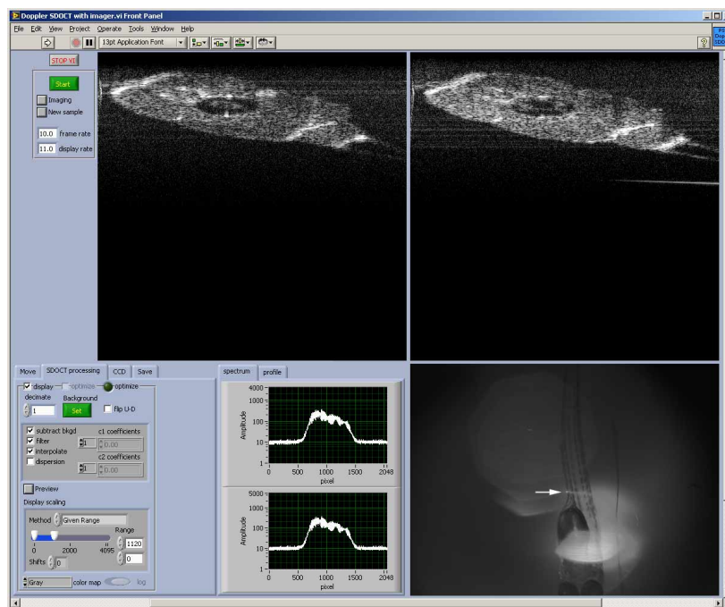
Fig. 4. Front panel of the acquisition software. OCT B-scan is across the tail just below the swim bladder. Arrow in the CCD image indicates position of the OCT line. (Aspect ratio of the scan is not 1.)
