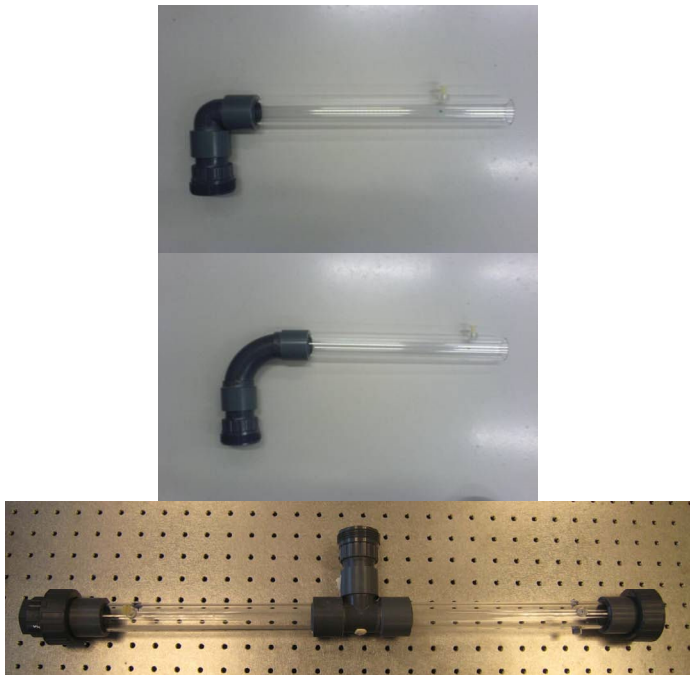
Figure 4: Three test geometries (Top left: Bend1, Top right: Bend2, bottom T-Joint).
