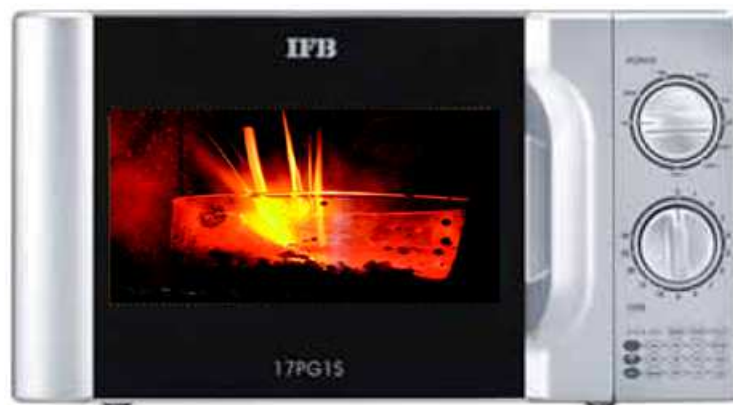
Fig. 4. Microwave oven for the powder synthesis.
