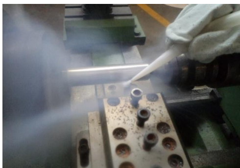
Fig. 2b. Cutting under Liquid N 2 Environment
