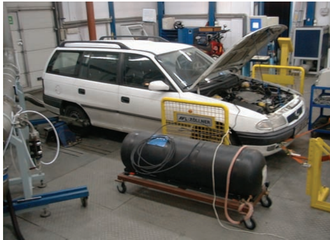
Fig. 1. Vehicle equipped with LPG systems tested at ITS as part of the statutory ITS work
