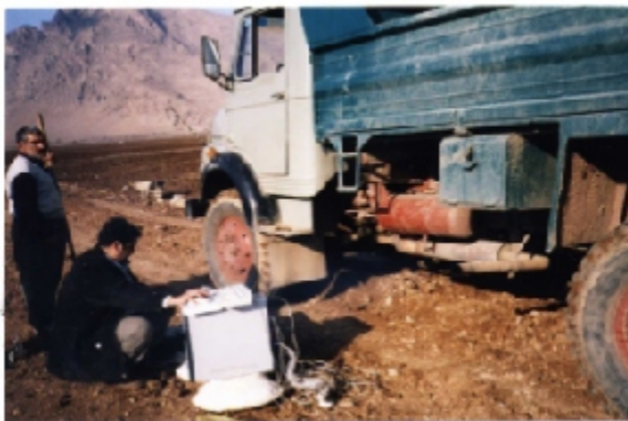
Fig. 10: Loading of truck on the pipe
