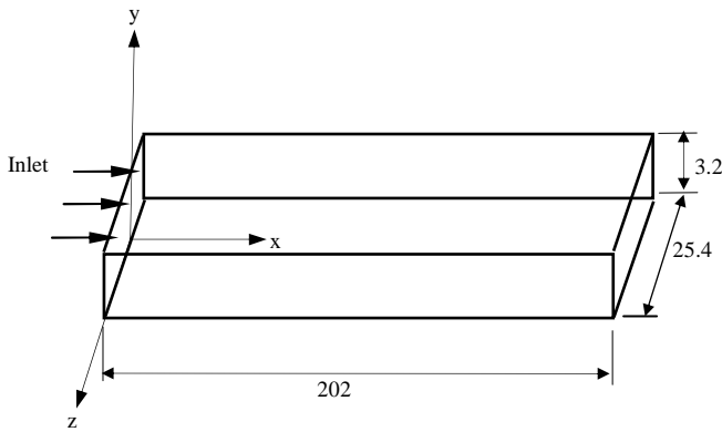
FIGURE 1. SCHEMATIC OF THE RECTANGULAR STRIP USED IN THE SIMULATION (ALL UNITS ARE IN mm).
