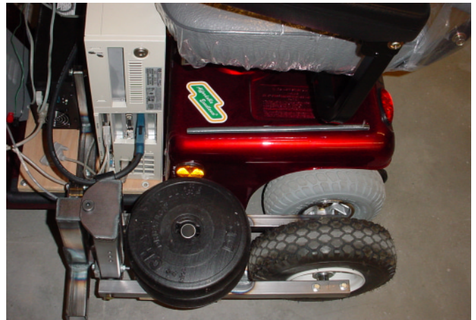
Fig. 15 Scooter equipped with instrumented redundant wheel
