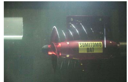
Figure 8 Cavitation at podded propulsor at DAT mode ( J=0.26 )
