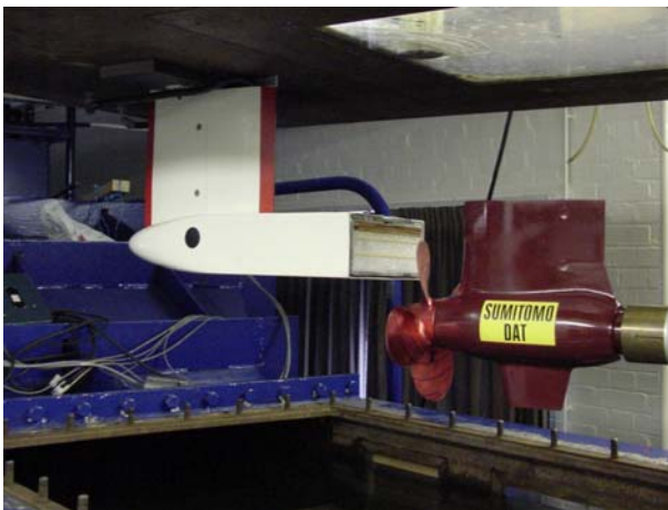
Figure 3 Ice milling mechanisms and model pod propulsor
