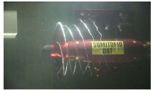
Figure 7 Cavitation at podded propulsor at bollard pull condition
