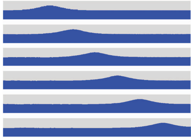
Fig. 2 Solitary wave propagation from free-surface elevation at t=0 s, t=2 s, t=4 s, t=6 s, t=8 s, and t=10 s.
