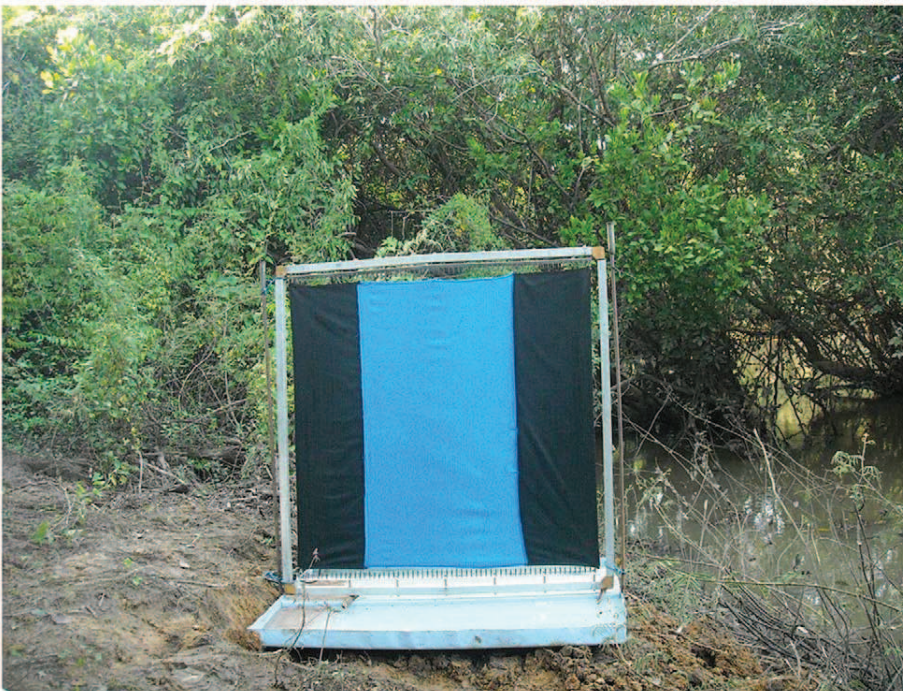
Figure 2. The standard 1 m×1 m Black Blue Black e-target (treatment A) set up on a tray. doi:10.1371/journal.pntd.0001332.g002
