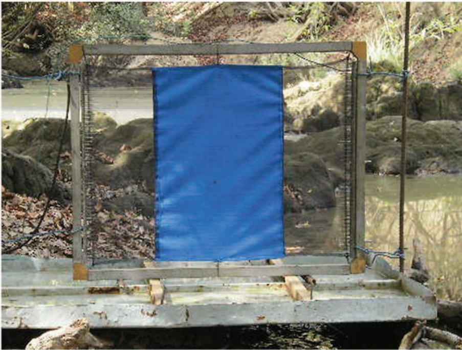
Figure 1. Example of a target design used for comparison. A 0.75 m wide×0.50 m high net-blue-net target (37.5 cm×50 cm blue surrounded by 2 pieces of net of 18.75 cm×50 cm each) inside an electric grid mounted on a fly collection tray. doi:10.1371/journal.pntd.0001332.g001
