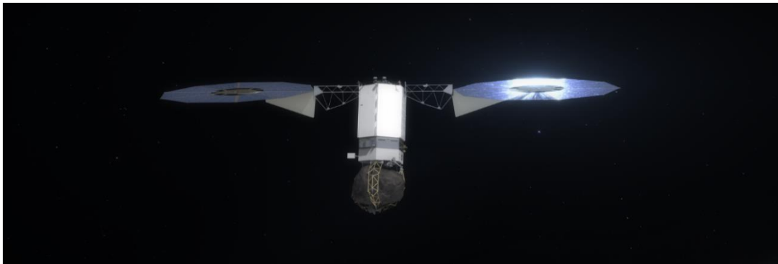
Figure 7: ARV with Captured and Restrained Boulder ready for EGT Operations (Image Credit: NASA/AMA, Inc.).
