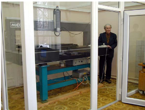
Fig. 1. The setup of the PAVICOM-1 system.
