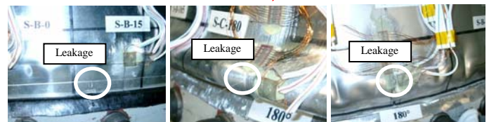
(Aluminum alloy) (Steel) (Stainless steel) Fig.7 Comparison of Ultimate State Level of Test Models
