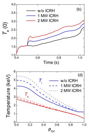
Figure 1. Time evolution of q-profiles (a) and central electron temperatures (b). q-profiles (c), ion and electron temperature profiles (d) and electron density profile (e) at 1.05 s for the without ICRH case, 1 MW ICRH case and 2 MW ICRH case
