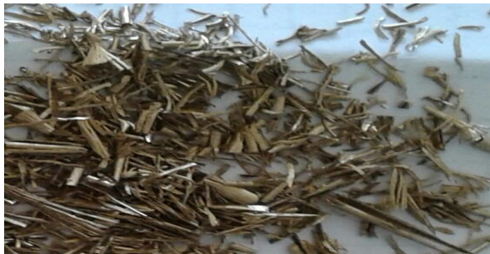
Figure 1: Photo of metallic fibers waste.
