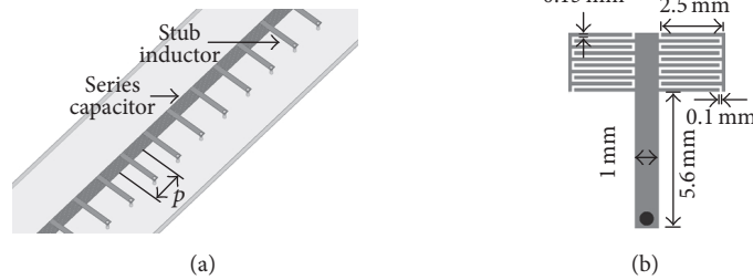
FIGURE 2: CRLH TL structures. (a) Periodic CRLH TLs with series capacitors and shunt stub inductors. (b) Geometry of unit cell of CRLH TL.
