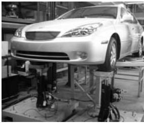
Fig 3: Shaker testing setup.
