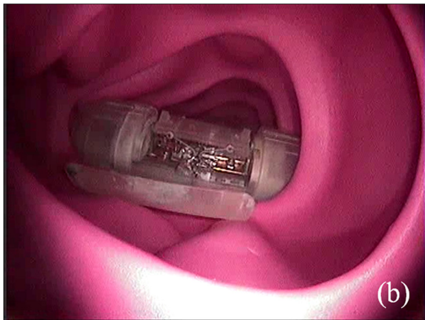
Fig. 12 PSP release test in GI phantom: robotic capsule, navigated to the target area, (a) prior to and (b) after PSP release
