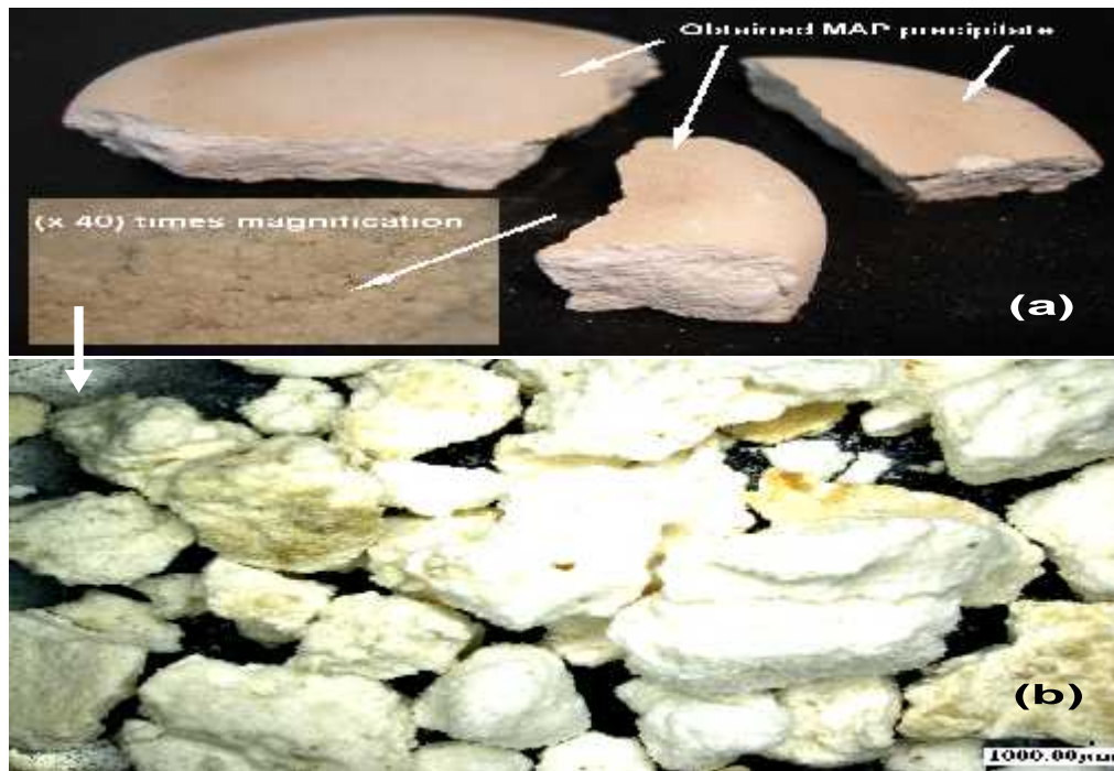
Fig. 2 Physical morphology of the original MAP product and 40 times magnification with stereo microscope.
