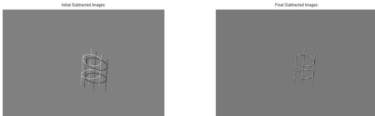
Figure 6. Geometrical matching algorithm. The left image is the FTRAC overlay with the \pm 10^\circ and \pm 10 mm random ground truth perturbation used to initialize the optimizer. The right image is the overlay after the geometrical matching algorithm has been executed.
