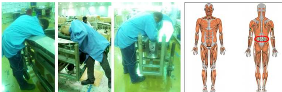
Fig. 1. Surface Electromyography instruments was setup to measure muscle fatigue in right and left thoracolumbar fascia muscle.
