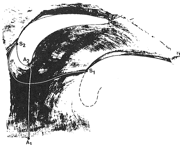
Fig. 3 Flow visualization of endwall (Goldstein and Chen, 1985)
