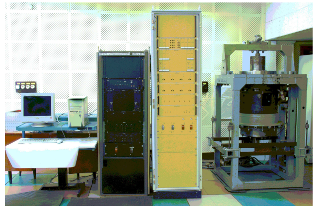
Figure 7 - Test facility for Radial EMB model
