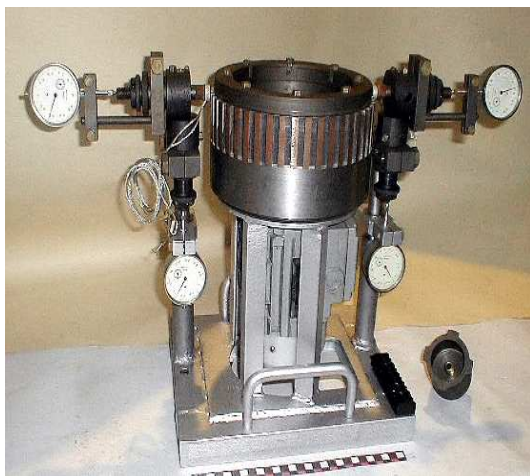
Figure 6 – Test facility for rotor EMB position sensors
