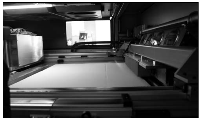
Fig. 8. Layer application in VoxelJet device chamber
