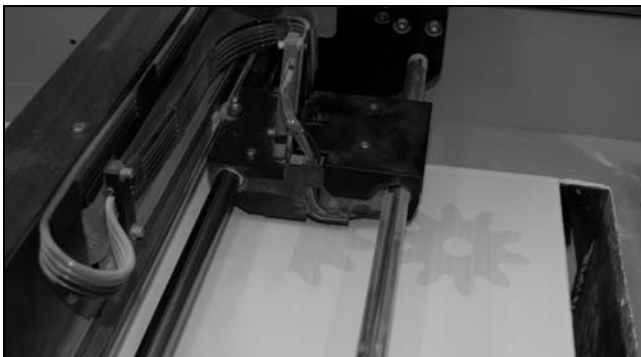
Fig. 6. Print out of model layer by 3DP method – Z510 Spectrum printer
