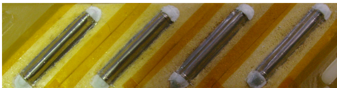
Figure 17b. Large scale ribbed model with four foam ribs encased in Inconel foil.
