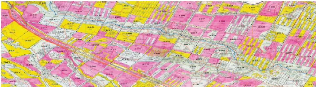
Fig.2 Classified ground-survey map, where the stands with red and yellow colors correspond respectively to those with damage more than 50% and less than 50% but greater than 30%.
