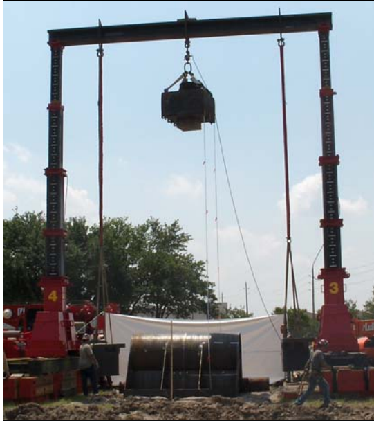
Figure 10 – Photographs of full-scale drop test set-up
