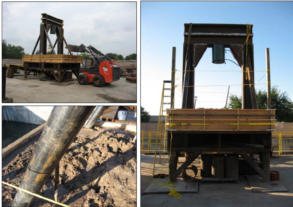
Figure 3 – Photographs showing vertical load frame
