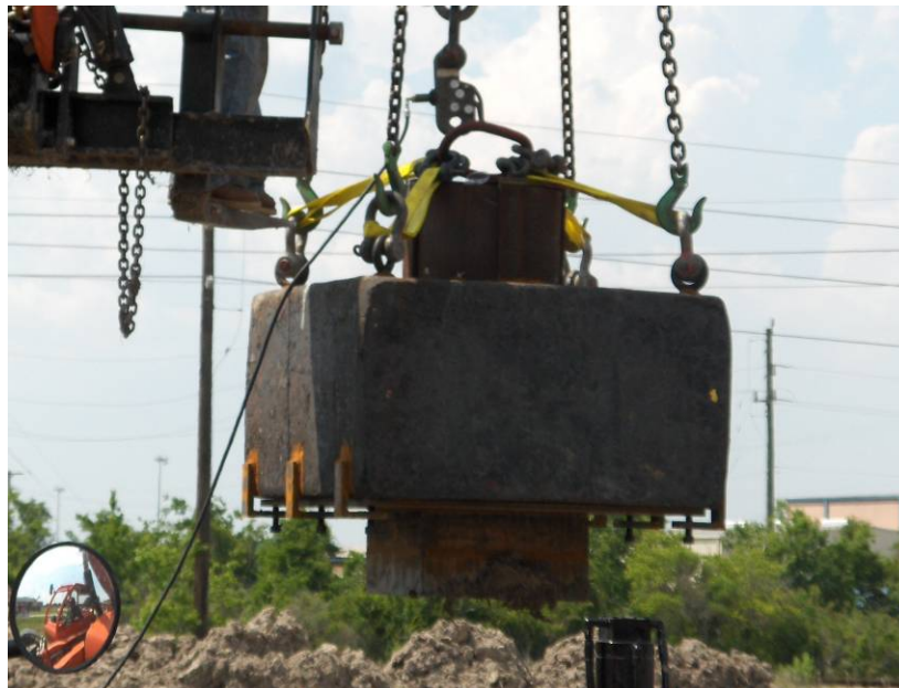
Figure 7 – Photograph of weight serving as dropped object
