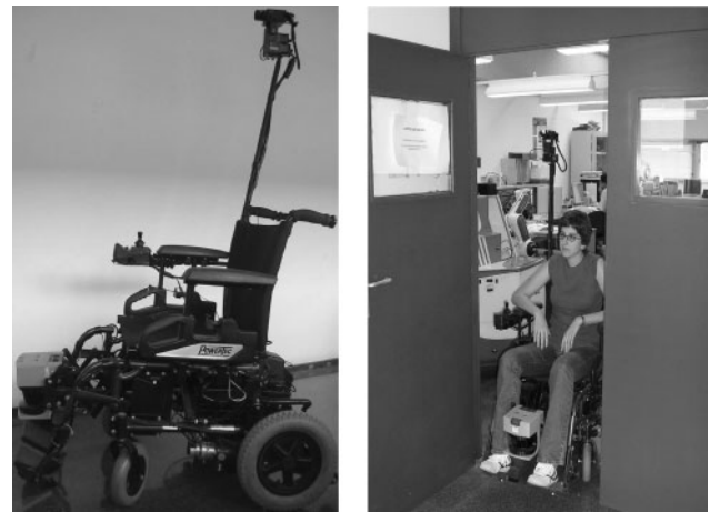
Figure 4 Two views of the SENA robotic wheelchair in which we have evaluated our human-robot integration architecture.
