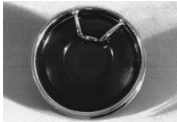
Fig. 1. Typical heart valve, where the occluder and minor strut are clearly visible.
