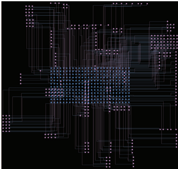
Fig. 4. RDL routing in TSV-whitespace style.
