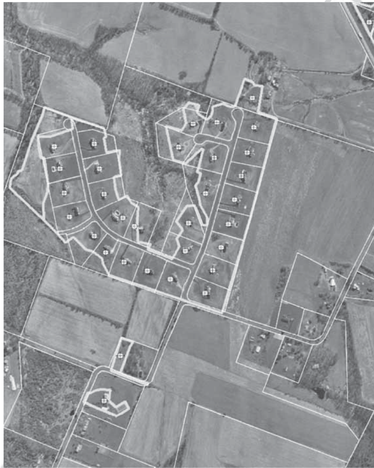
39 40 41 42 43 Figure 6.7 Housing unit location automation. This image depicts an orthophoto of one newly developed housing tract. The thick lines delineate the 'patches' of new urban growth as classified by the land use/land cover dataset. The thin lines delineate the property parcel lines. The target symbol denotes the automated centroid location estimated for each new housing unit. Sprawl measurements are calculated for each housing unit centroid
