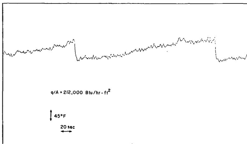
Fig. 10 Test heater temperature trace during run 25
