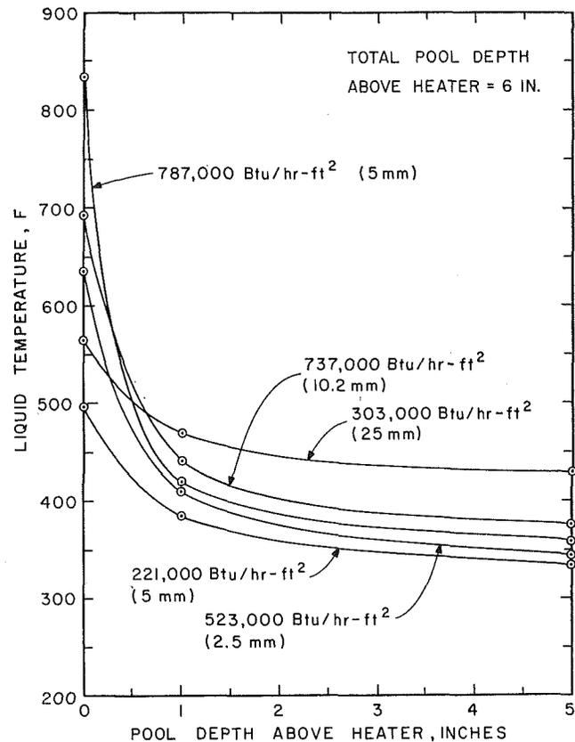
Fig. 12 Pool temperature gradients
