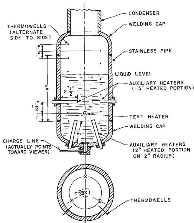
Fig. 2 Boiling vessel
