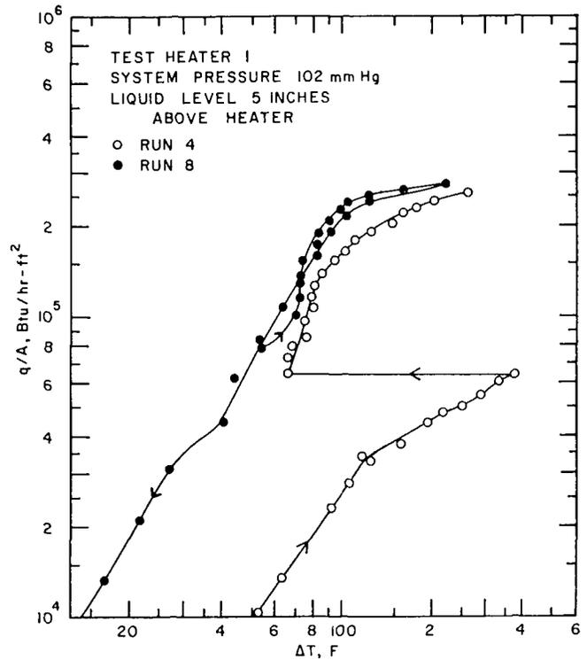
Fig. 9 Effects of aging on test heater 1
