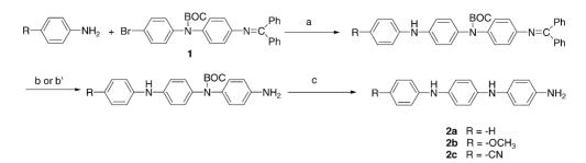
Fig. 1. Synthesis of substituted trimeric anilines. Key: (a) Pd(OAc)<sub>2</sub>, DPEphos, NaOt-Bu, toluene, 110 °C, 24 h; (b) R: -H,  $-OCH_3$ : Pd/C, NH<sub>4</sub>HCO<sub>2</sub>, THF/MeOH, 60 °C, 24 h; (b') R: -CN: HONH<sub>2</sub>, pyridine, CHCl<sub>3</sub>/THF/EtOH, 3 h; (c) 180 °C, 10 h.
