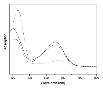
Fig. 3. UV-vis spectra of oxidized trimers in DMF, (1) solid line: APPBD; (2) dash line: APMBD; and (3) dot line: APCBD.
