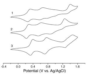
Fig. 4. Cyclic voltammagram of (1) APPBD; (2) APMBD; and (3) APCBD, measured in tetrabutylammonium perchlorate (0.1 M) in acetonitrile with a scan rate of 100 mV/s.
