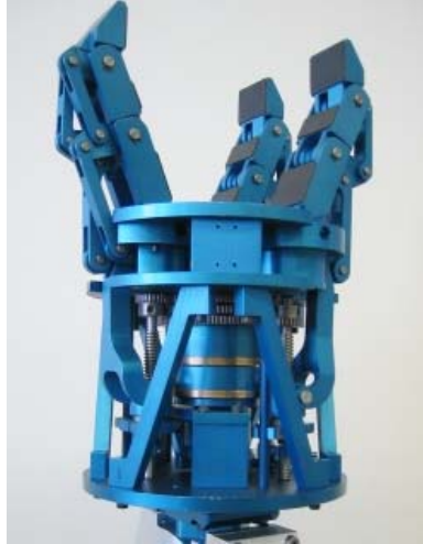
Figure 3. University of Laval End-Effector using coupled planetary system
