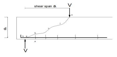
Figure 6: Crack development in beams
