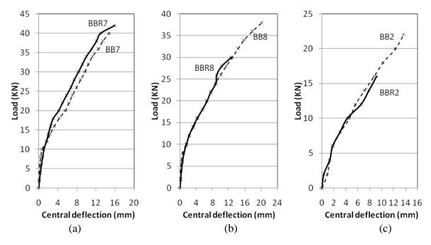
Figure 4: Typical load deflection curves of tested beam
