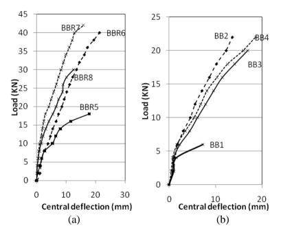
Figure 5: Comparison of different web reinforcement
