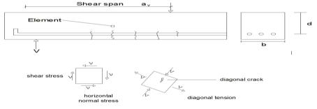
Figure 2: Stresses on an element in concrete beam
